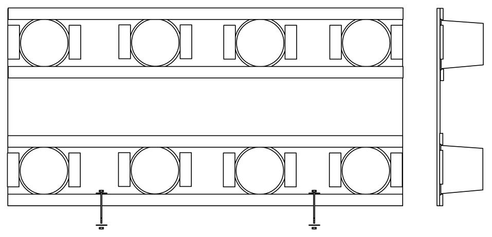
NOTE 1. The plastic buckets can be deformed to snap into Ithe retianers. and several buckets may bed stacked to add height to the stage.
